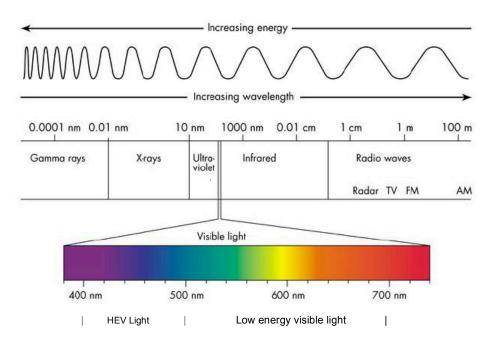
The human eye responds to only a small portion of the entire electromagnetic energy spectrum the portion described as the visible light spectrum.
